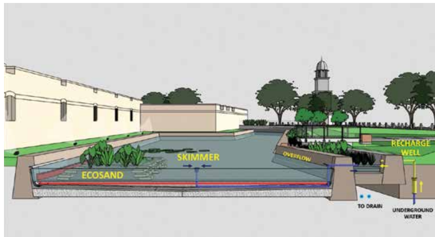
The hybrid filtration system makes use of aggregate filters inside the water basin and a plant-based bio-retention swale between the moat and the outer glacis.
